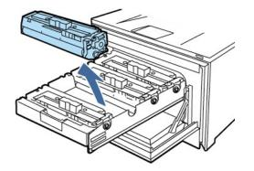
4. Remove the new toner cartridge package from the box, and then pull the release tab on the packaging.
