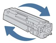
7. Do not touch the imaging drum on the bottom of the toner cartridge. Fingerprints on the imaging drum can cause print-quality problems. Also, do not expose the cartridge to light unnecessarily.
