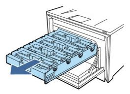
3. Grasp the handle on the toner cartridge, and then pull the toner cartridge straight up to remove it.
