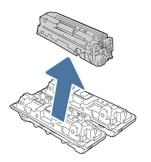
6. Hold both ends of the toner cartridge and rock it end to end to distribute the toner evenly inside the cartridge.
