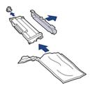
7. Hold the toner cartridge by the handle and shake it from left to right several times, as shown. Then push it firmly into the drum unit until it locks into place.
