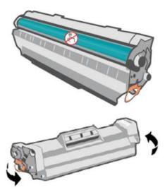
5. Bend the orange tab until it snaps, and then pull to remove the sealing tape from the cartridge.
