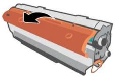
4. Grasp the cartridge by its sides, and then rock the cartridge side to side five or six times to evenly distribute the toner.
